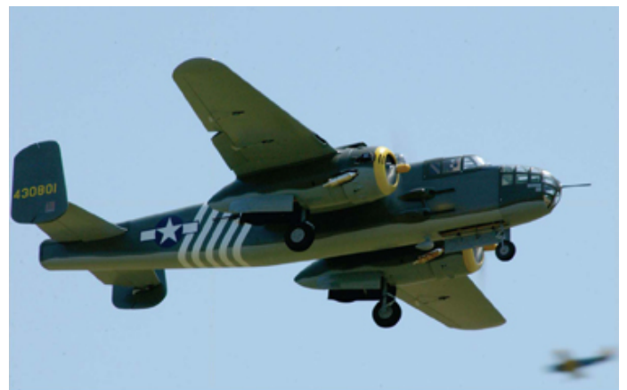
The Top Flite B-25 Mitchell bomber has inboard and outboard flaps and lands like a trainer.
